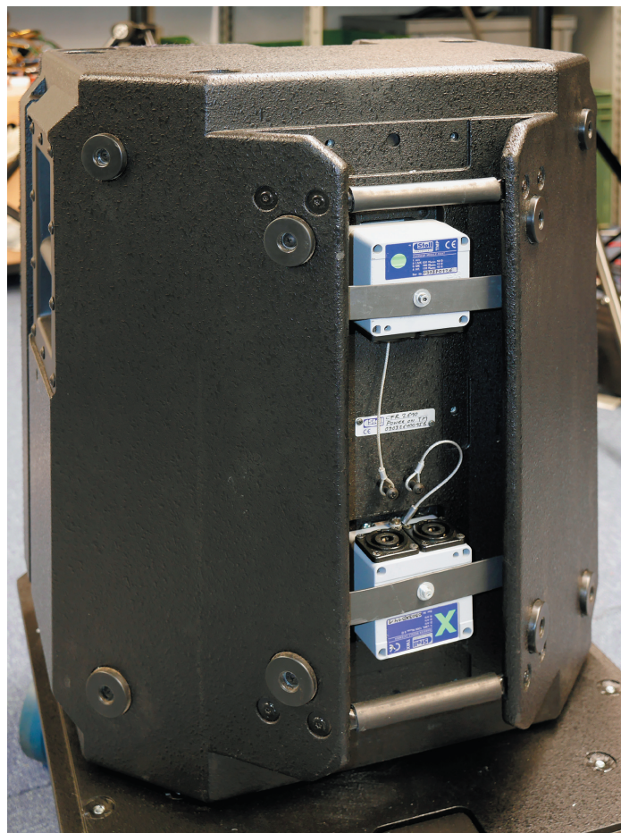
Front and back of the Stoll CFR2610 Convertible. The transfer modules with Speakon connectors are easily discernible on the back.
